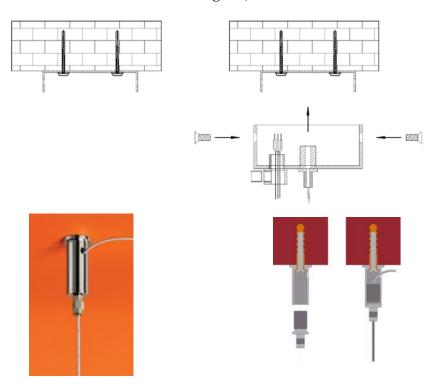
Attach to the ceiling hanger from ceiling rose and suspension holders. Then connect the power cables to the terminals. NOTE !!! Luminaires with the option of dimming have additional terminal marked with "+" and "-". After connecting cables, apply ceiling rose body and fasten it with moles. You can now attach the main voltage.
